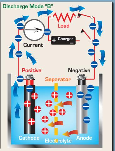
Negative ion and positive electron flow in charge mode "A" and discharge mode "B"
