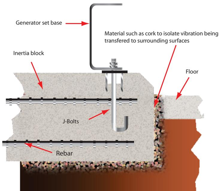
Diagram 4 - Section of spring vibration isolator mounting
